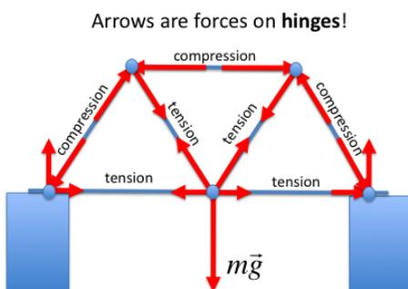
To create longer beams, bridge designers add supporting lattice work, or a truss, to the bridge's beam. This support truss adds rigidity to the existing beam, greatly increasing its ability to dissipate the compression and tension. Once the beam begins to compress, the force is dissipated through the truss.
