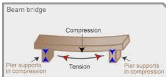
**Compression:** The force of compression manifests itself on the top side of the beam bridge's deck (or roadway). This causes the upper portion of the deck to shorten.
