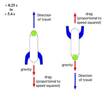
In this phase of its flight, the only forces acting on the rocket are gravity, and the aerodynamic drag force.
