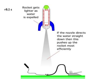
Just under half the water has now left the rocket. The rocket has reached a height of around 0.5 meters and is travelling upwards at approximately 10 meters per second. This corresponds to very large acceleration of around 100 meters per second per second, or roughly 10g.
