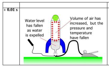
As the catch is released, the gas pushes the water out through the nozzle, and the rocket begins to lift off. The pressure of the air begins to fall, and also its temperature drops as the air expands.
