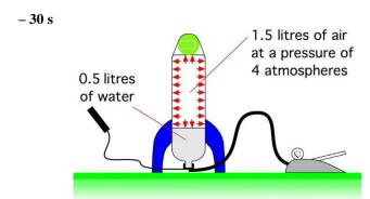
Your chosen launch pressure is reached. To be specific, we'll assume that the gauge on the foot pump you have used reads 3 atmospheres. Since the pressure before you started was one atmosphere the actual pressure of the air in the bottle is now 4 atmospheres. 1 atmosphere – sometimes called 1 bar, is roughly equivalent to:
