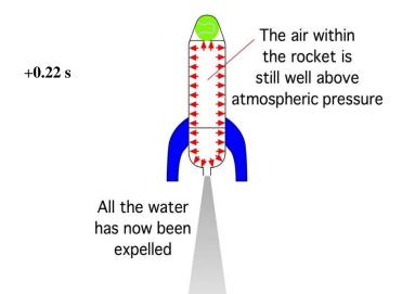
Amazingly all the water has now left the rocket. If you could just imagine emptying 500 ml of water out of a bottle it might easily take 10 seconds. It has now all gone in just under a quarter of a second! The rocket is now travelling at around 26 metres per second.
