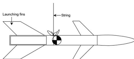
This position of the string marks the center of gravity. Measure this position on the rocket (fuel should be present)
