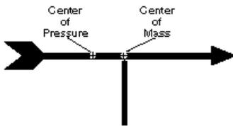
The reason that the weather vane arrow points into the wind is that the tail of the arrow has a much larger surface area than the arrowhead. The flowing air imparts a greater force to the tail than the head, and therefore the tail is pushed away. There is a point on the arrow where the surface area is the same on one side as the other. This spot is called the center of pressure.
